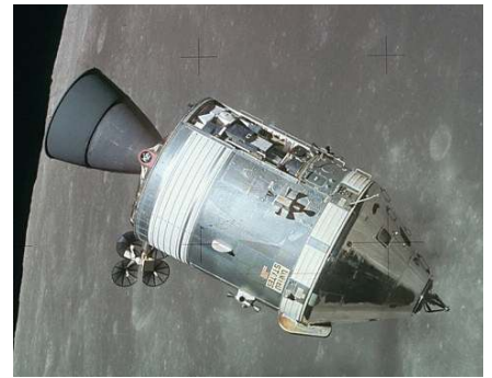
Command and Service Modules of Apollo 15 (Apollo 11's was the same). NASA
